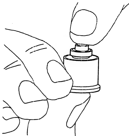
Fig. 42 Delivery valve inspection
